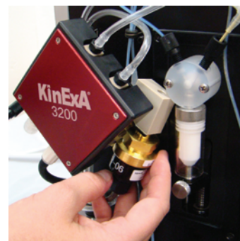
Figure 3. Removing the pressure transducer from the mount.
