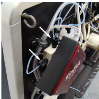
Figure 1. Plumbing attached to the pressure transducer block.
