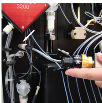
Figure 4. Pulling the connector through the hole.
