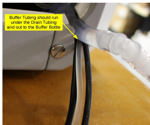
Figure 3: Drain and Buffer Lines exiting the Instrument.
