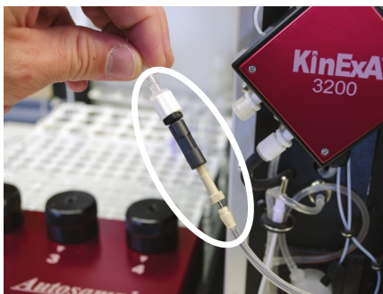
Figure 2. Connecting the Autosampler and KinExA Buffer Lines.
